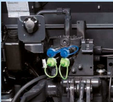
The **5 Series** can be equipped with up to five remote valves. Three valves are mechanically operated by levers integrated into the right-hand console. Two additional mid-mount remotes are available as an option for the use of L Series front loaders or other front-mounted implements.
